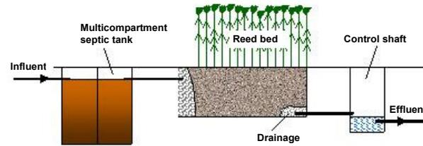
Fig. 5: Schematic diagram of horizontal filter (Source: TBW GmbH)
