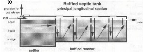
**Fig. 4: Schematic diagram of baffled septic tank (Source: [7])**
