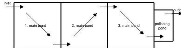
Fig. 7: Flow pattern of aerobic-facultative ponds in series
