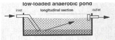
Fig. 6: Anaerobic ponds (Source: [7])
