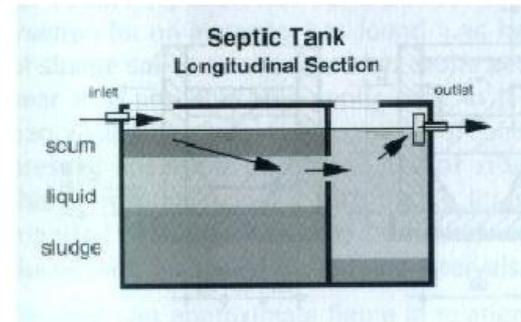
Fig. 1: Schematic diagram of septic tank
