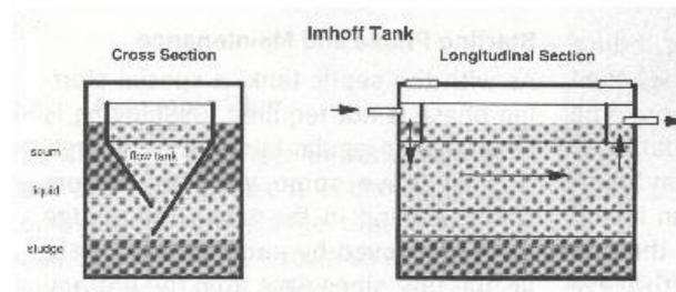
Fig. 2: Schematic diagram of Imhoff tank (Source: [7])
