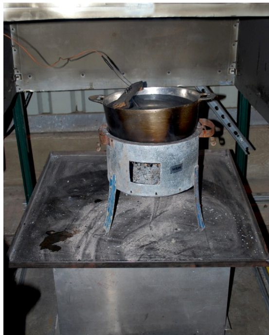
Fig. 1b: Above: The stove testing system at LBNL. Below: A close-up view of a stove (the Mirak) on the testing platform, with the front doors of the exhaust hood open to view the set-up.
